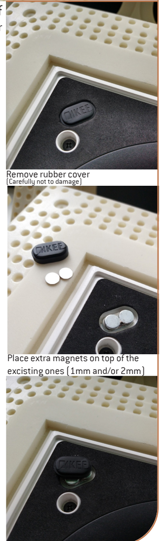
Installation of K_CI160QS_Cover
